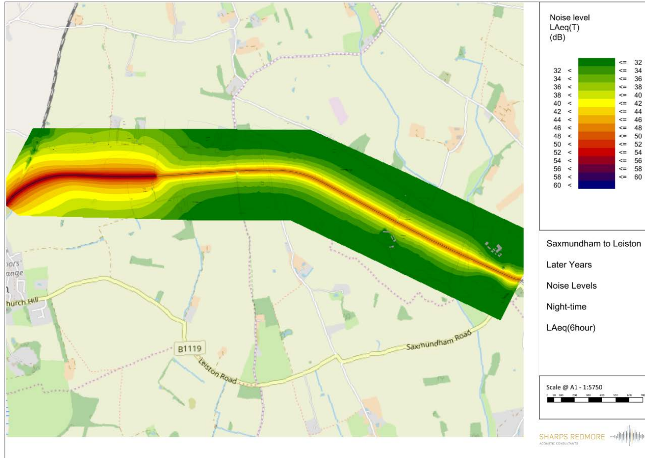
Figure 9.3.C.2: Saxmundham to Leiston – Later Years – Night – 7 train passes – Branch Line Section, L Aeq , 6 h
