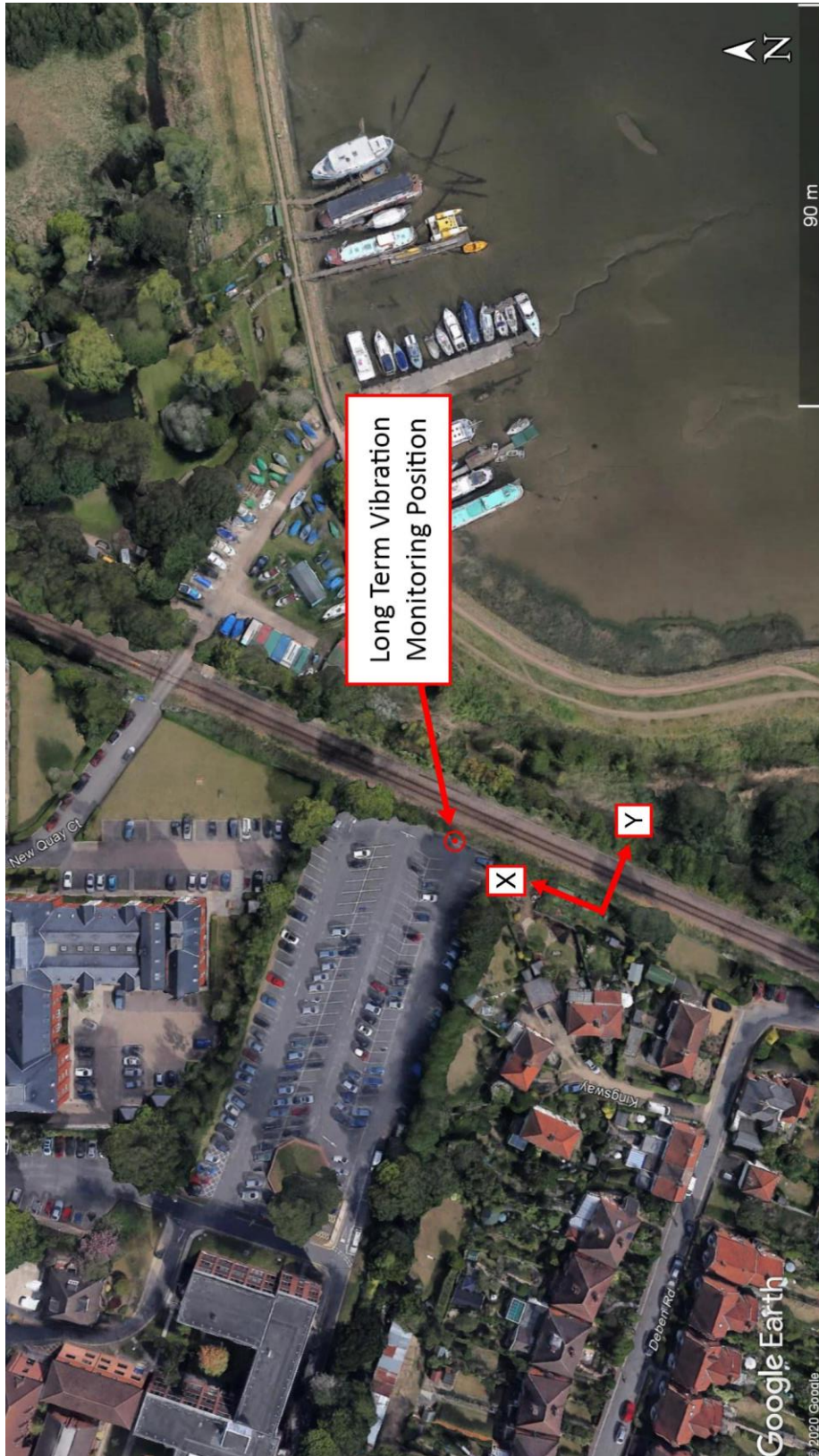
Figure A1: Plan showing vibration monitoring location
