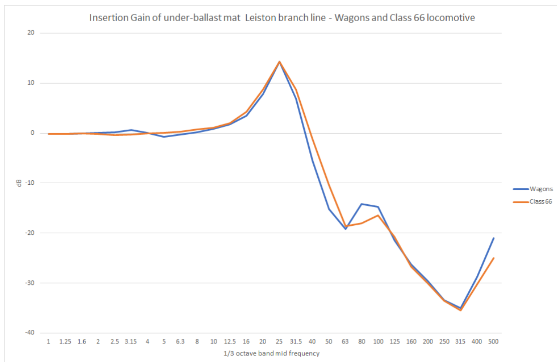
Figure 8 Insertion gain of Getzner under-ballast mat
