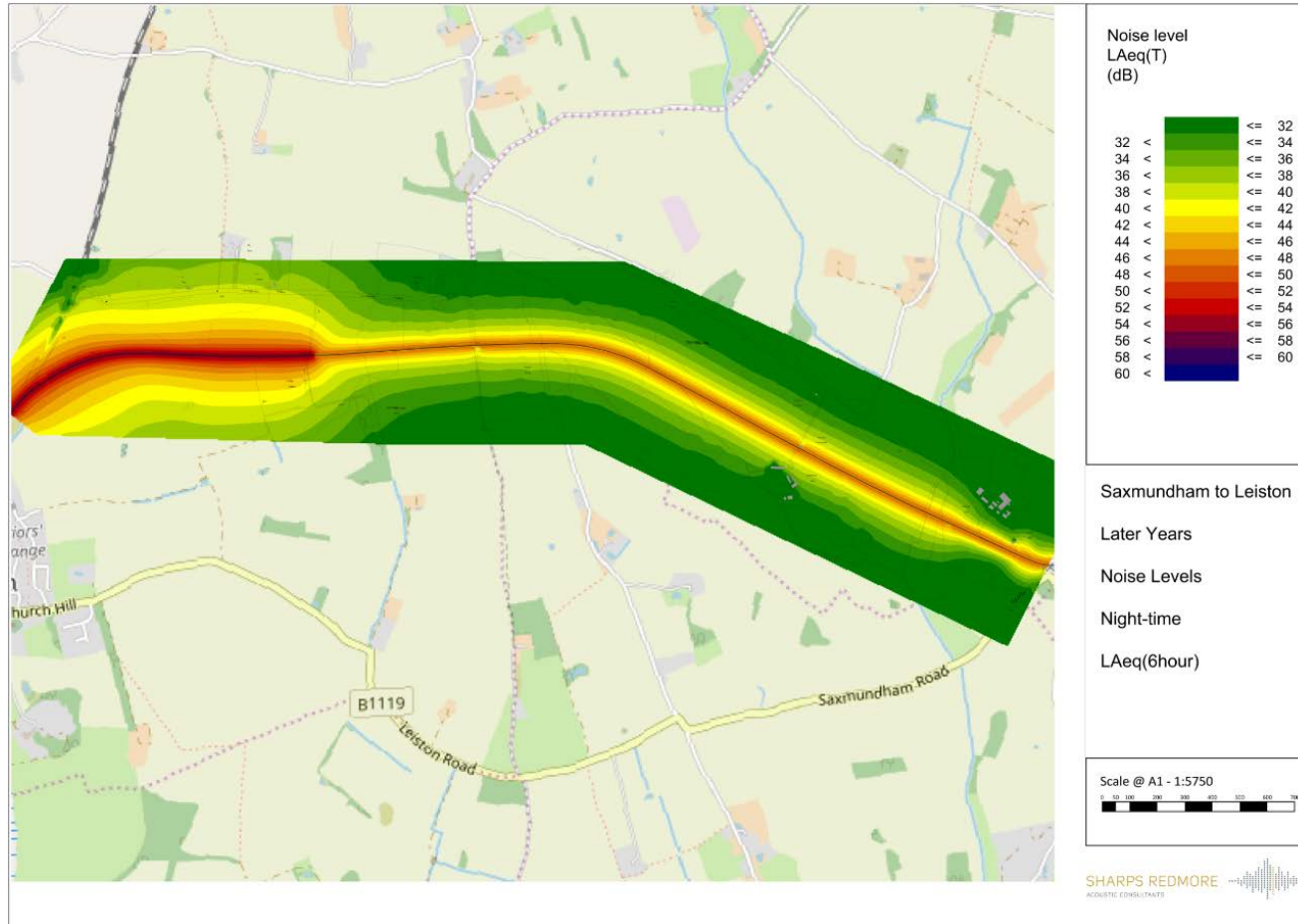
Figure 9.3.C.3: Saxmundham to Leiston – Later Years – Night 8 train passes – Branch Line Section, L_{Aeq, 6h}
