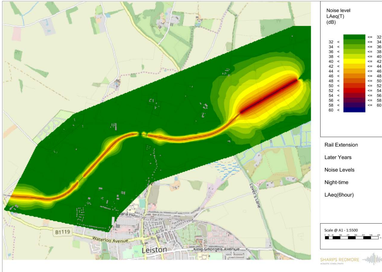
Figure 9.3.C.6: Rail Extension Route – Later Years – Night – 8 train passes – Branch Line Section, LAeq, 6 h
