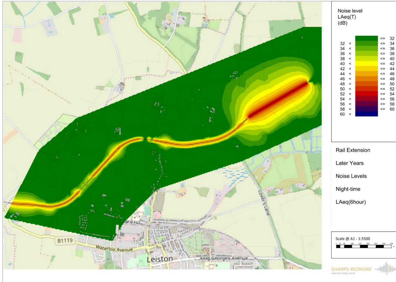
Figure 9.3.C.5: Rail Extension Route – Later Years – Night – 7 train passes – Branch Line Section, LAeq, 6 h
